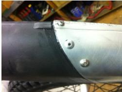
Fit both front pipe & silencer with new o-rings and silicone sealer.
